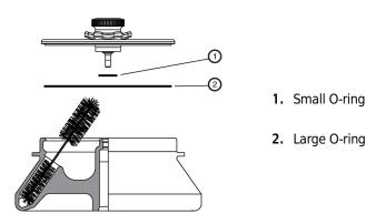
**6** Clean metal threads every 6 months, or as necessary. Use a brush and concentrated Solution 555.
