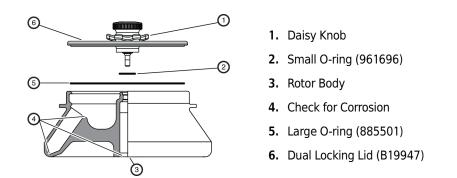
**NOTE** Do not use sharp tools on the rotor that could cause scratches in the rotor surface. Corrosion begins in scratches and may open fissures in the rotor with continued use.
