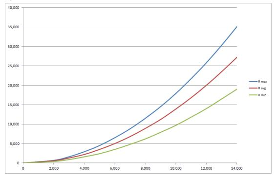
Figure 9 Relative Centrifugal Fields Chart for the JA-14.50 Rotor
